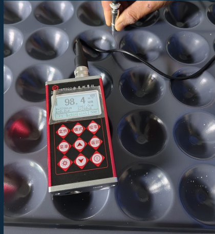
Panel coating thickness
